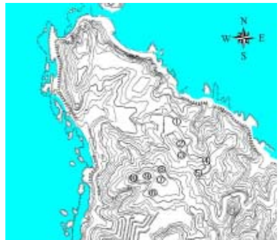
Figure 2: Contour map of TAPPI Wind Park. Encircled numbers - indicate the turbine locations.
